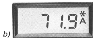
Fig. 2.5. a) Battery depleted b) Maximum L_{eq} duration exceeded
